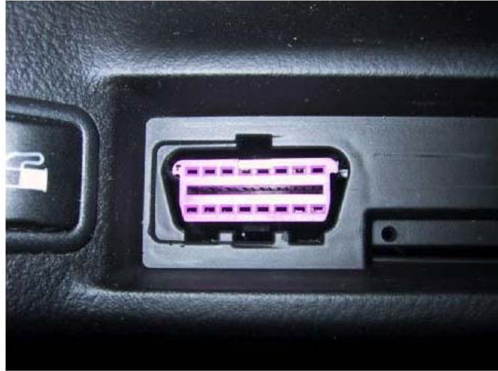
DLC located between front seats near parking brake under rubber cover.
